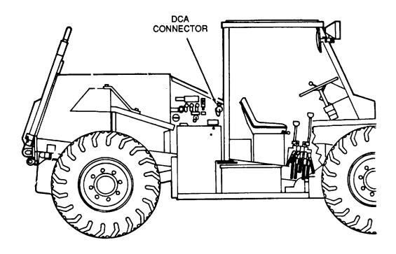
Figure 2-2. Vehicle DCA Connector
