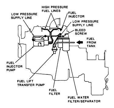
Figure 1-7. Engine Fuel System Components
