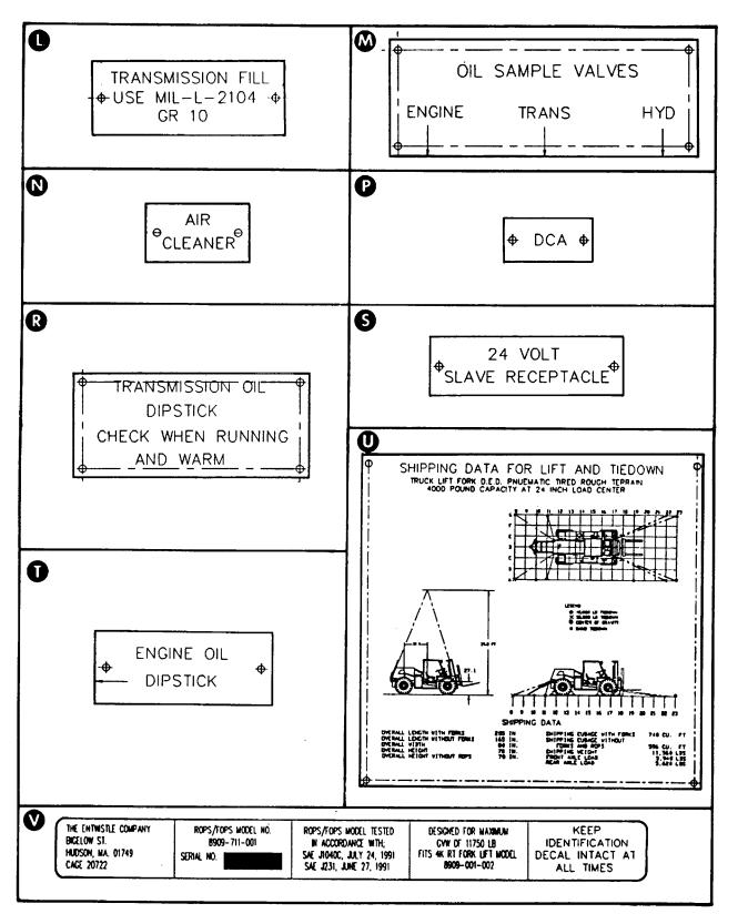
Figure 1-4. Forklift Truck Information Plates and Stencils (Sheet 5)
