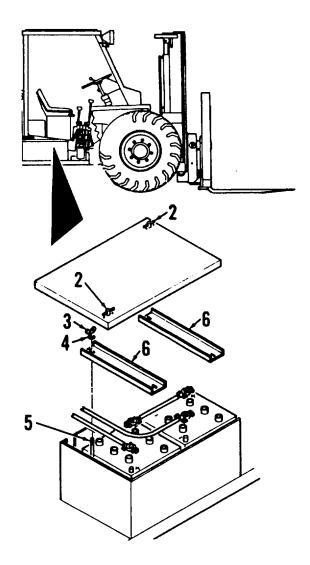
3. Drive pin (7) out of lid latch (2). Remove lid latch from battery box lid (1) by removing screws (8) and nuts (9).
