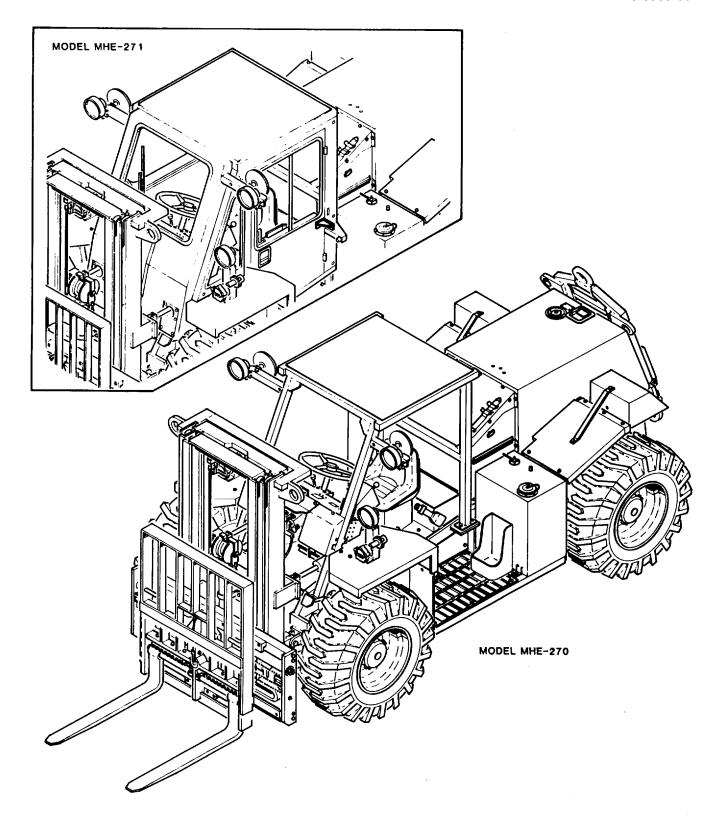
Figure 1-1. 4000 Pound Capacity Rough Terrain Forklift Truck, Models MHE-270 and MHE-271
