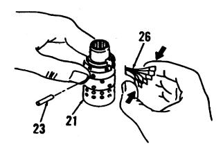
Position spool and sleeve assembly (21) so that splined end of spool enters 15 hole end of housing.
