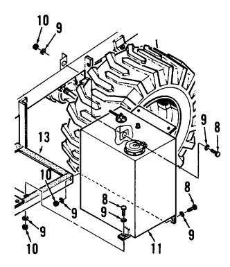
2. Inspect three neoprene rubber pads (13) for damage, deterioration, or permanent set. Replace pads as required.
