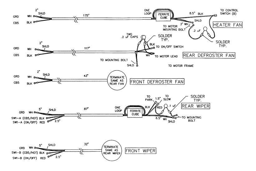
Figure FO-5. Cab Wiring Harness
