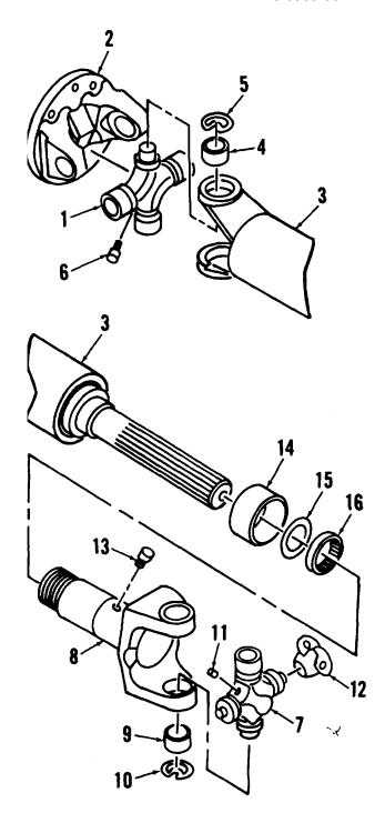
15. Remove grease fitting (13) from slip yoke (8) only if replacement is required.
