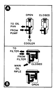
Figure 1-9. Engine Lubricating System Components
