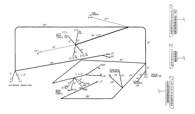
Figure FO-3. Main Wiring Harness (Sheet 1 of 3)
