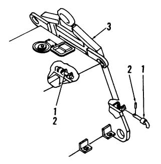
Install tow bar latch pins (1) using spring pins (2).
