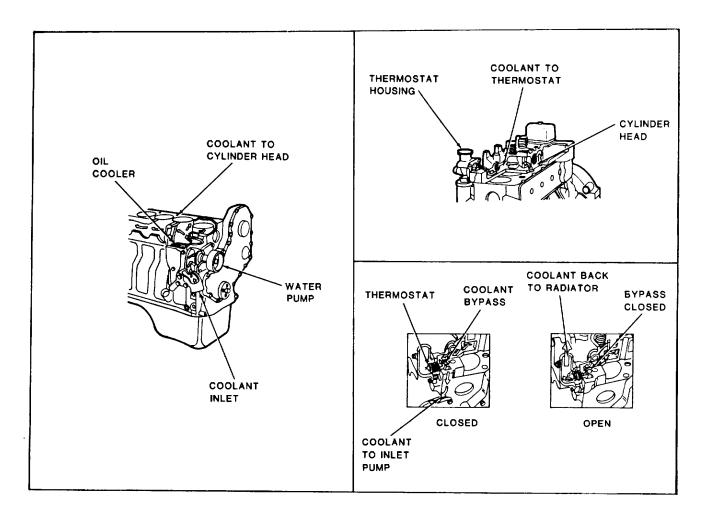
Figure 1-8. Engine Coolant System Components
