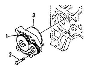
10. If installing a new oil pump, measure gear backlash (dimensions D AND E). Backlash limits for D and E shall be 0.003 TO 0.013 in. (0.08 TO 0.33 mm).
