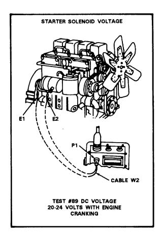
Trouble Symptom 2. Engine Cranks But Will Not Start, No Smoke From Exhaust
