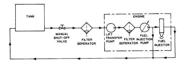
Figure 1-6. Fuel System Schematic
