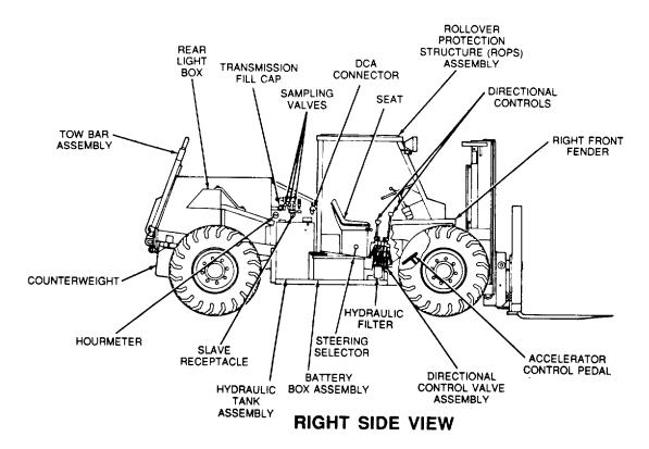
Figure 1-2. Forklift Assemblies and Major Components
