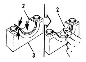
3. Install lower bearing halves (1) onto journals in cylinder block. Ensure tangs on bearing halves set into notches in journals. Lubricate bearings with Lubricate 105.
