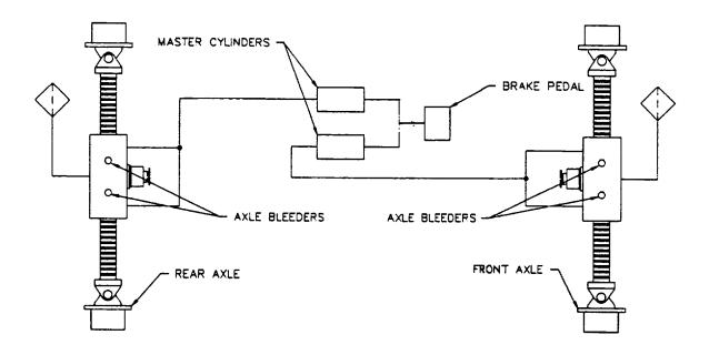
Figure 1-12. Brake System Schematic
