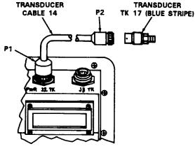
INSTALL TRANSDUCER INTO TUBE TO PIPE **ADAPTER**
