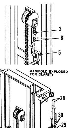
5. Measure distance between top of inner rail (26) and top of outer rail (31) on both sides. Distance shall be 1.0 inch. If required, adjust mainlift chains as follows:
