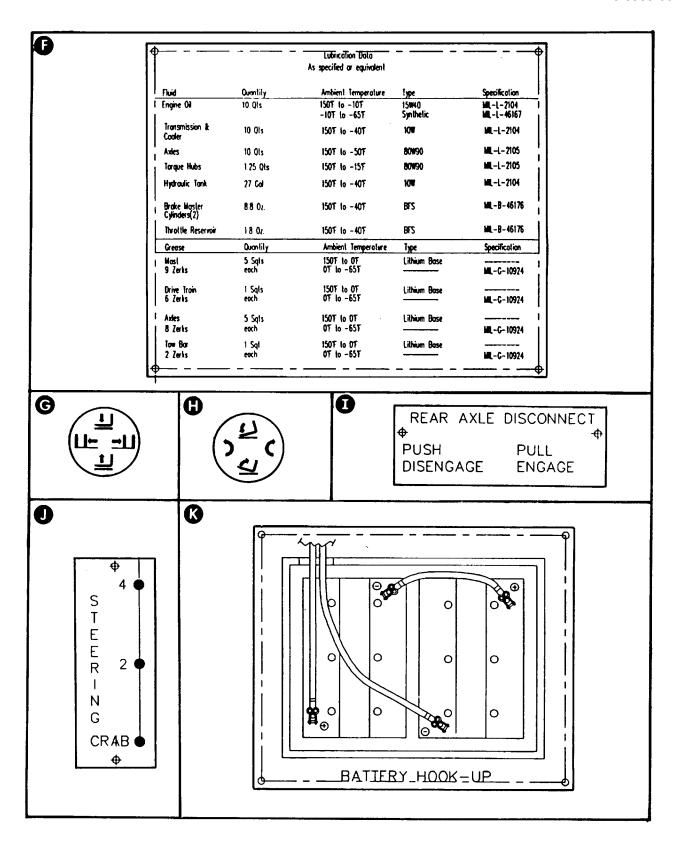
Figure 1-4. Forklift Truck Information Plates and Stencils (Sheet 3)
