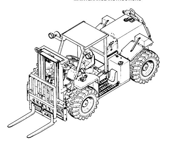
TRUCK, FORKLIFT, 4000 LB CAPACITY ROUGH TERRAIN, DED, PNEUMATIC TIRE
