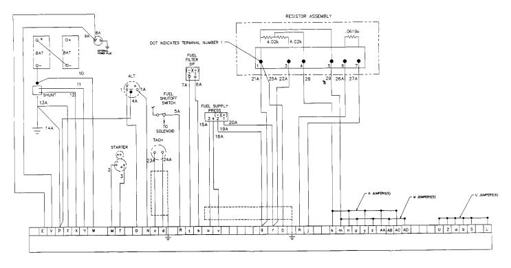
Figure FO-4. DCA Wiring Harness
