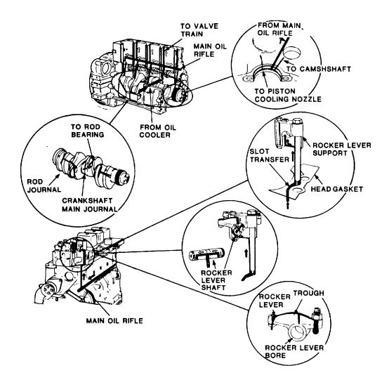
Figure 1-10. Power Component Lubrication
